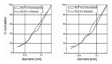
Figure 7. Grading curves for 2 samples of material with frictional-viscous behavior.
