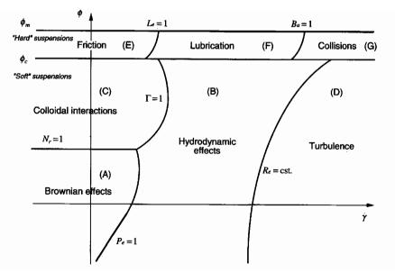
Figure 1. Simplified diagram of flow regimes, where Pe = Péclet number, Nr = repulsion number,  $\Gamma = a$  ratio between viscous and colloidal interactions, Re = Reynolds number, Le = Leigthon number, Ba = Bagnold number,  $\phi_m =$  the maximum random solid concentration and  $\phi_c =$  the minimum concentration for a network of particles in close contact to form (for more details see Coussot & Ancey 1999).
