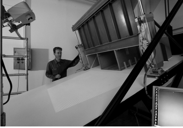
Figure 3. View on the sluice gate and the reservoir at the channel inlet.
