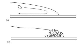
Fig. 19. Schematic of the behavior contrast beween fine-grained and coarsegrained flows. (a) Conveyer-belt-like flow at the front and (b) formation of a frictional front. After [188].
