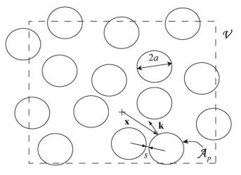
Fig. 9. Idealized suspension of spherical particles in a Newtonian fluid.
