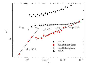
Fig. 16. Variation in the dimensionless torque  $M = C/(\pi \rho' gh R_1^3)$  (where *C* is the measured torque) exerted on the vane by the tested suspension as a function of the rotational speed  $\Gamma$ . For material features, see Table 2. After [6].
