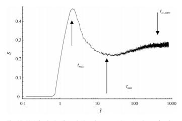
Fig. 17. Variation in the dimensionless shear stress  $S = \tau/(\bar{\rho}gh)$  as a function of dimensionless time  $\tilde{t} = t\Omega$ . Experiments made for a suspension made up of glass beads ( $\phi_c = 0.589$ , a = 0.4 mm), kaolin ( $\phi_k = 0.098$ ,  $\tau_c = 1.2$  Pa), and water ( $\phi_t = 0.629$ ). After [6].
