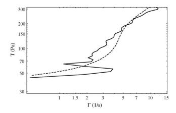
Fig. 15. Flow curve for 1 mm beads within a water–glycerol solution ( $\phi = 0.605, \mu_0 = 1.05$  Pa s). The solid line represents the WVD solution, while the dashed line represents the Tikhonov solution. After [7].
