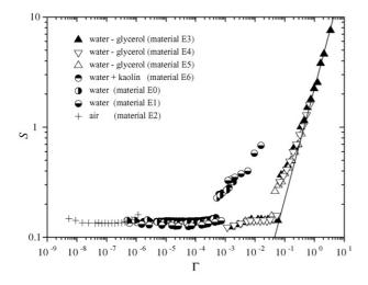
Fig. 13. Variation in the dimensionless shear stress as a function of the dimensionless number  $\Gamma$ . The line slope is unity and indicates a linear variation of *S* with  $\Gamma$ . The features of each material are specified in Table 2. After [6,9].
