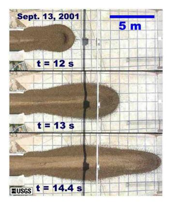
Fig. 20. Snapshots showing slurry flow discharging from the U.S. Geological Survey Debris-flow Flume and crossing the unconfined, nearly horizontal runout zone. The dark-toned material around the perimeter of the flow was predominantly gravel, while the light-toned material in the center of the flow was liquified mud. Figure reproduced from [127]; courtesy of Dr. R.M. Iverson.
