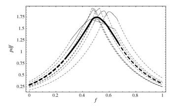
Fig. 28. Empirical probability distribution functions (pdf) of the 173 *f* values collected from the seven paths. The thick line represents the distribution function of the total sample, whereas the thin lines are related to individual paths. Each curve has been split into three parts: the central part (solid line) corresponds to the range of computed  $\mu$  values, while the end parts have been extrapolated. After [8].
