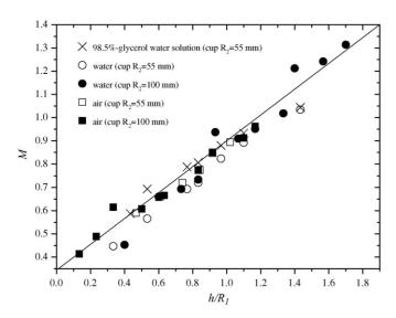
Fig. 14. Variation in the reduced torque  $M = C/(\pi \bar{\rho}' g h R_1^2)$  as a function of the scaled flow depth  $h/R_1$ , with  $R_1$  the inner cylinder radius. After [6,9].
