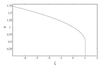
Fig. 23. Flow-depth profile of the viscoplastic simple wave generated after the wall is removed. Computations made with  $K = 4 \text{ m}^{-1} \text{ s}^{-1}$  and  $h_p = 1 \text{ m}$ .
